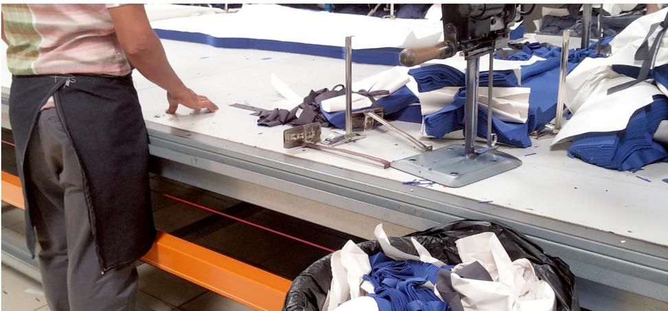
**Cutting tables at the cut & sew facility:** constantly cut out a stack of fabric generating various types and shapes of offcuts. The high speed pressure leaves the cut marking paper pieces and fabric go into the bin without separation.
