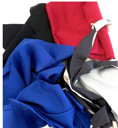
High-Press Fibre Panel comes in various sizes, density and thickness to cater for different purposes from wall panel, roof insulation, flooring, etc. (left), polyester offcuts are the only material that makes this versatile panel (right)
