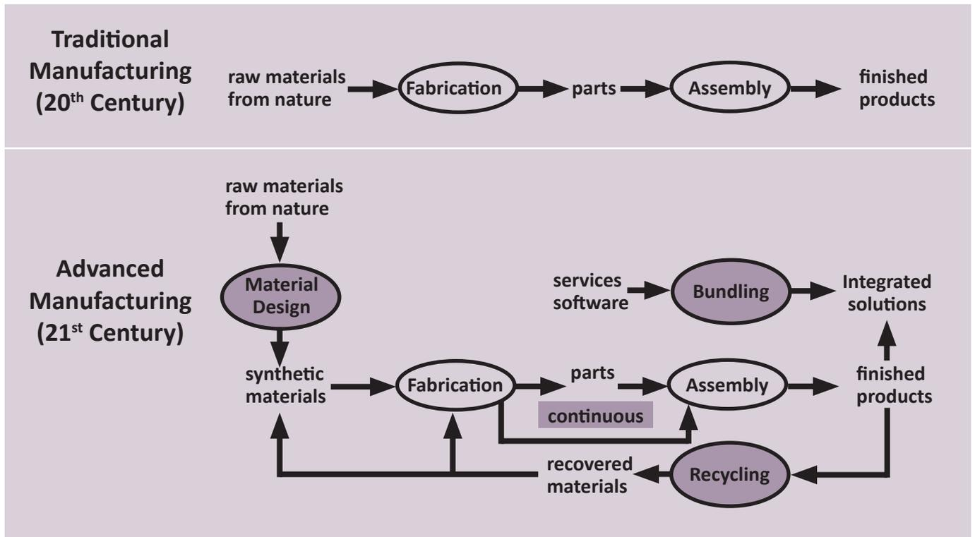
**FIGURE 1:** Definition of advanced manufacturing (bottom) as an expansion of traditional manufacturing (top) (De Weck and Reed, 2014).
