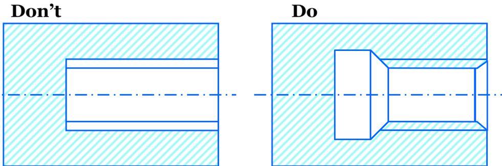
**DO - Provide an undercut for threads in turned components**
