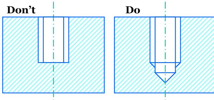
**DO - Design holes to the shape of the tool. If a hole is to be tapped, provide space for it.**
